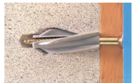
Fig. 31: Minimum screw length.
